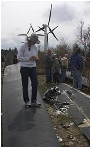
■ One of two turbine blades struck by lightning remains at the Searsburg wind plant and is a curiosity to visitors.
